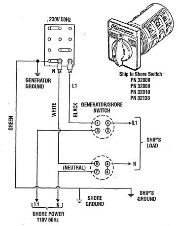
SHORE POWER NOTE: Diagram shows connections for a two-wire, 120 volt system. For a three-wire system, use the dotted lines
