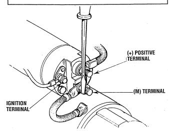
Test again by jumping the two large terminal studs. Hold the screwdriver blade firmly between the studs. Do not allow the screwdriver blade to touch the solenoid or starter casing, this would cause a short.
