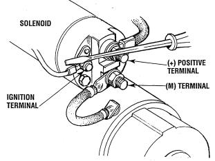
If nothing happens at all, the solenoid is not getting current.. Check the battery isolation switch and inspect the wiring connections. it is also possible that the solenoid is defective.
