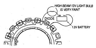
Reverse the leads across the diode. The diode should block voltage passing through it, and the headlight should not glow, or it may glow faintly.
