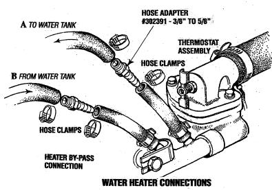
Using the Heater By-Pass connection, install hoses A and B as illustrated below. Use the hose adapters (PN 302391) to increase the hose size from 3/8" to 5/8".
