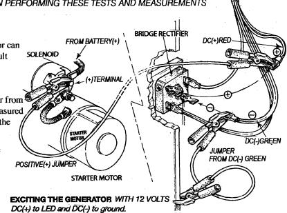
C(+) to LED and DC(-) to ground. #4 Keeping the EXCITER CIRCUIT polarity correct. FRAME
