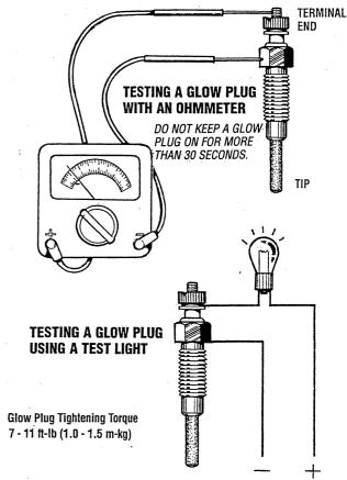
Re-install the plugs in the engine and test them again. The plugs should get very hot (at the terminal end) within 7 to 15 seconds. If the plugs don't heat up quickly, check for a short circuit. When reinstalling the glow plugs, use anti-seize compound on the threads.
